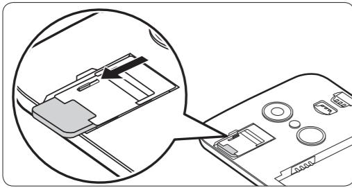
To remove the SIM Card from Slot 1, push the pin at the top to the left.
